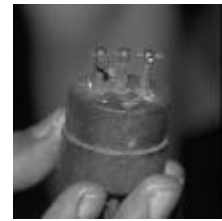
Figures 5b and 5c. A closeup of the spark gaps normally mounted inside the transmitting antenna.
