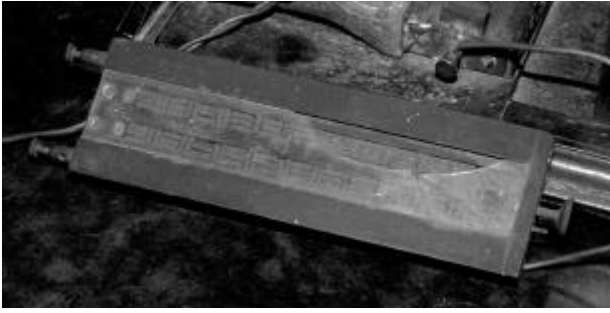
Figure 13. One of Bose's free-space radiation receivers, recently described [11] as a "space-irradiated multi-contact semiconductor (using the natural oxide of the springs)." The springs are kept in place in their tray by a sheet of glass, seen to be partly broken in this photograph.
