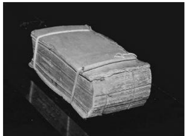
Figure 7. One of Bose's polarisers was a cutoff metal-plate grating, consisting of a book (Bradshaw's Railway Timetable) with sheets of tinfoil interleaved within the pages.
