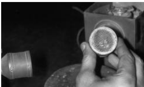
Figure 5a. One of Bose's transmitter antennas (being held on the right of the picture). Note the polarising grid; the spark gap is just visible behind the grid. In the background behind this antenna, part of the high voltage equipment used to generate the spark can be seen. At the left of the picture is the receiving horn.
