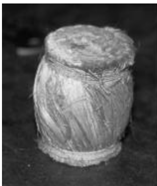
Figure 9. One of the twisted-jute polarisers used by Bose.
