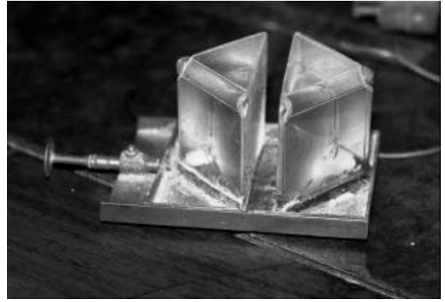
Figure 15. One of Bose's original double-prism attenuators, with adjustable air gap.
