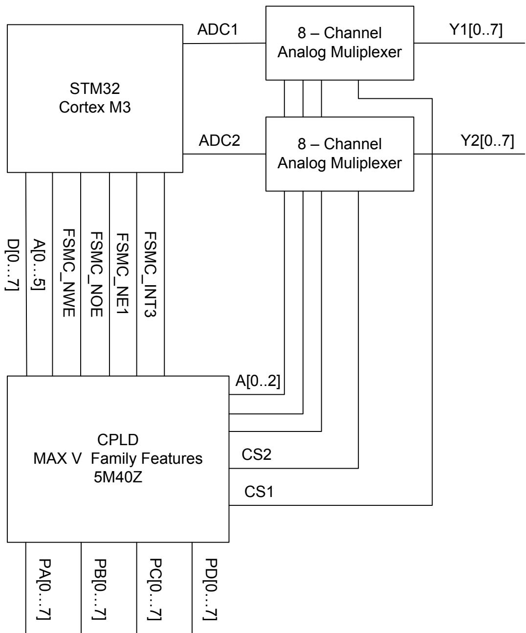
FSMC – Flexible static memory controller
