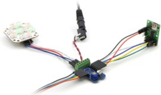
Connecting the Micro Maestro to a chain of ShiftBars. A single 12V supply powers all of the devices.
