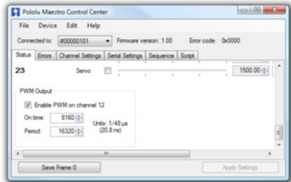
The PWM Output control in the Status tab in the Maestro Control Center (only available on the Mini Maestro 12, 18, and 24).
