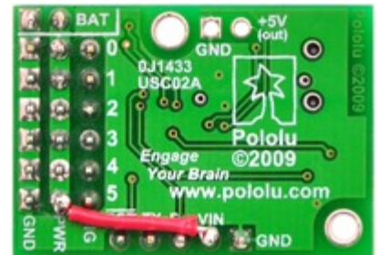
Micro Maestro configured to use a single power supply for both board and servos.
