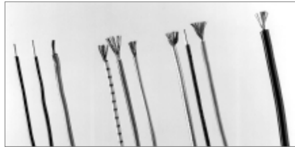
Fig. 139 Types of wire used in luminaires.From left to right: solid core (3),stranded (3),with heat-resistant insulation (3) and high-voltage ignition cable (1).
