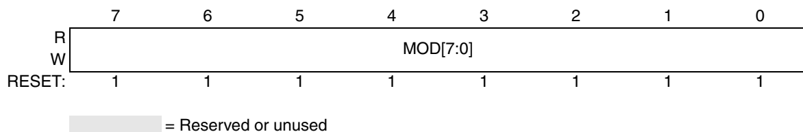
Figure 17-11. PDB Modulus Register Low (PDBMODL)
