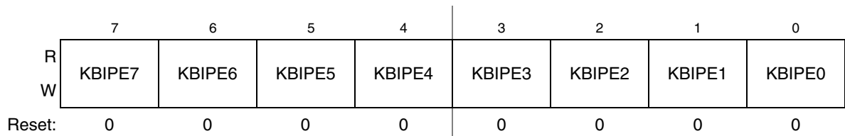
Figure 7-3. KBIx Pin Enable Register
