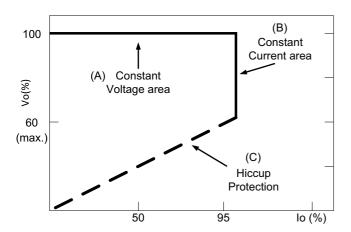
Typical LED power supply I-V curve
