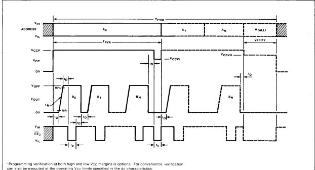
can also be executed at the operating V<sub>CC</sub> limits specified in the dc characteristics.
