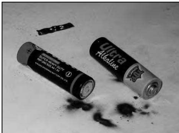
How do we use this to join two batteries to each other? First the items we need for this: the batteries and a little strip of metal for the 'solder tag' (a piece from a tin can or such works well).
