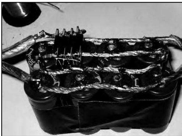
The MOSFETs. We had no need for blown up PCBs, so we built the prototype on top of the capacitors 'in the air'.
