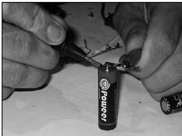
Attach the tag to one welding electrode and gently push it against the battery. Then push the other electrode firmly against the metal next to the tag and brace yourself for the flash.
