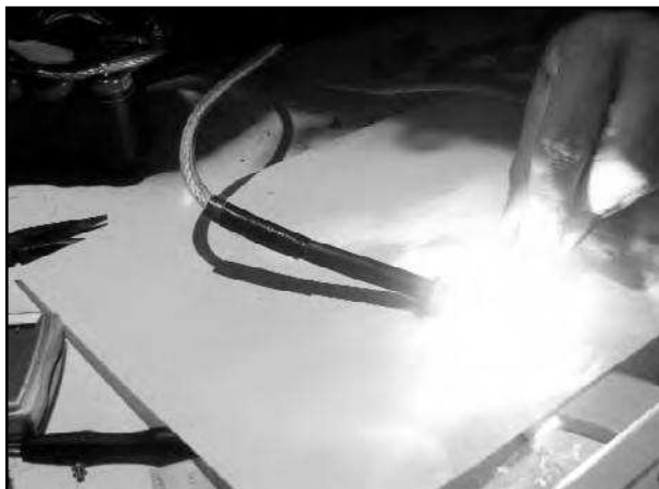
The first test: drawing sparks! It appears that the capacitor array can get rid of its power fast. Be aware of small pieces of metal shooting away.
