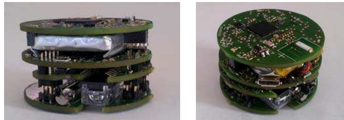
Fig. 14. Second prototype of the microrobot (a) lateral view, (b) angle view.
