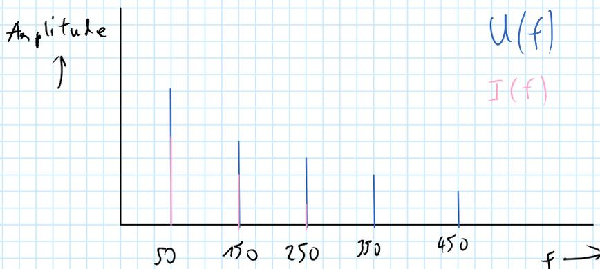
$$R = \frac{U(50\text{Hz})}{I(50\text{Hz})} \quad Z$$
