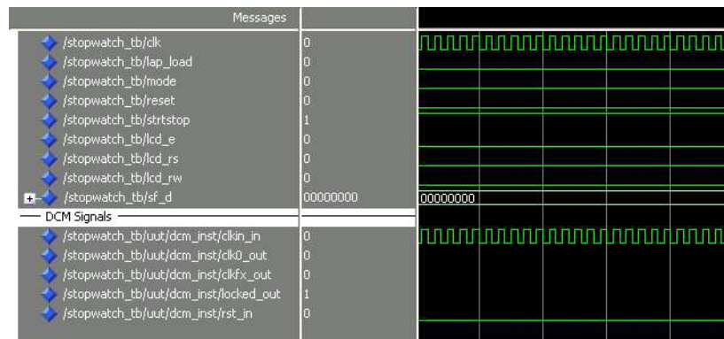
Figure 5-6: Waveform After Adding DCM Signals Divider
