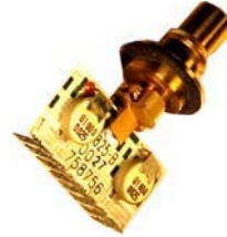
Gripper nozzle with a hybrid circuit
