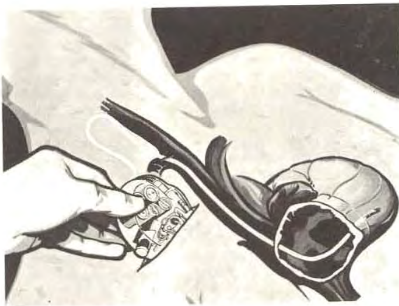
Fig. 4-24 A potentiometer provides adjustment of electrical output of implanted heart pacer
