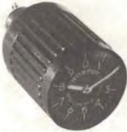
Fig. 3-26 A multiturn dial with a clocklike scale
