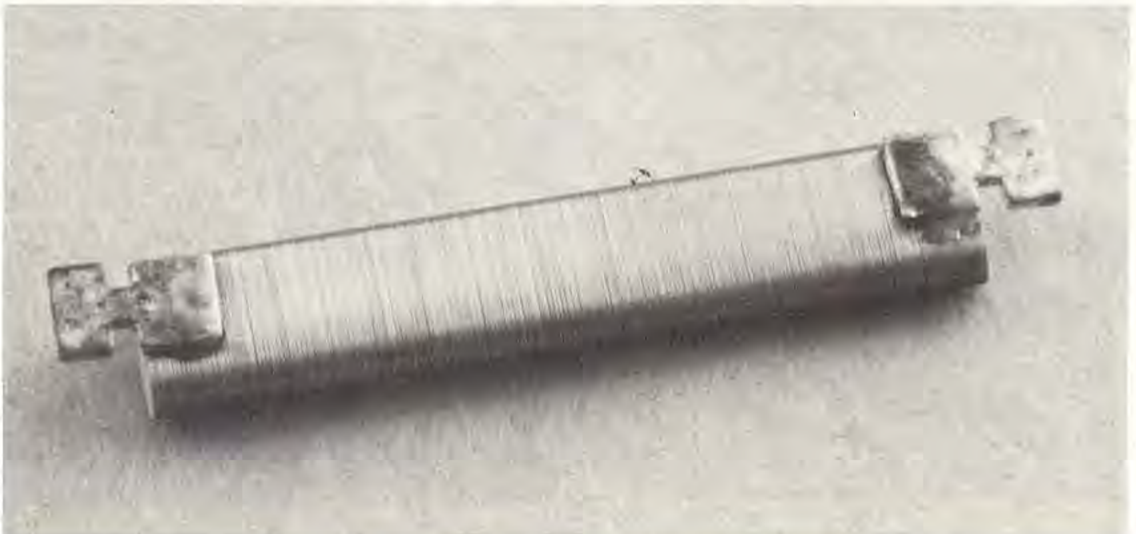
Fig. 2-26 Linear wirewound potentiometer element
