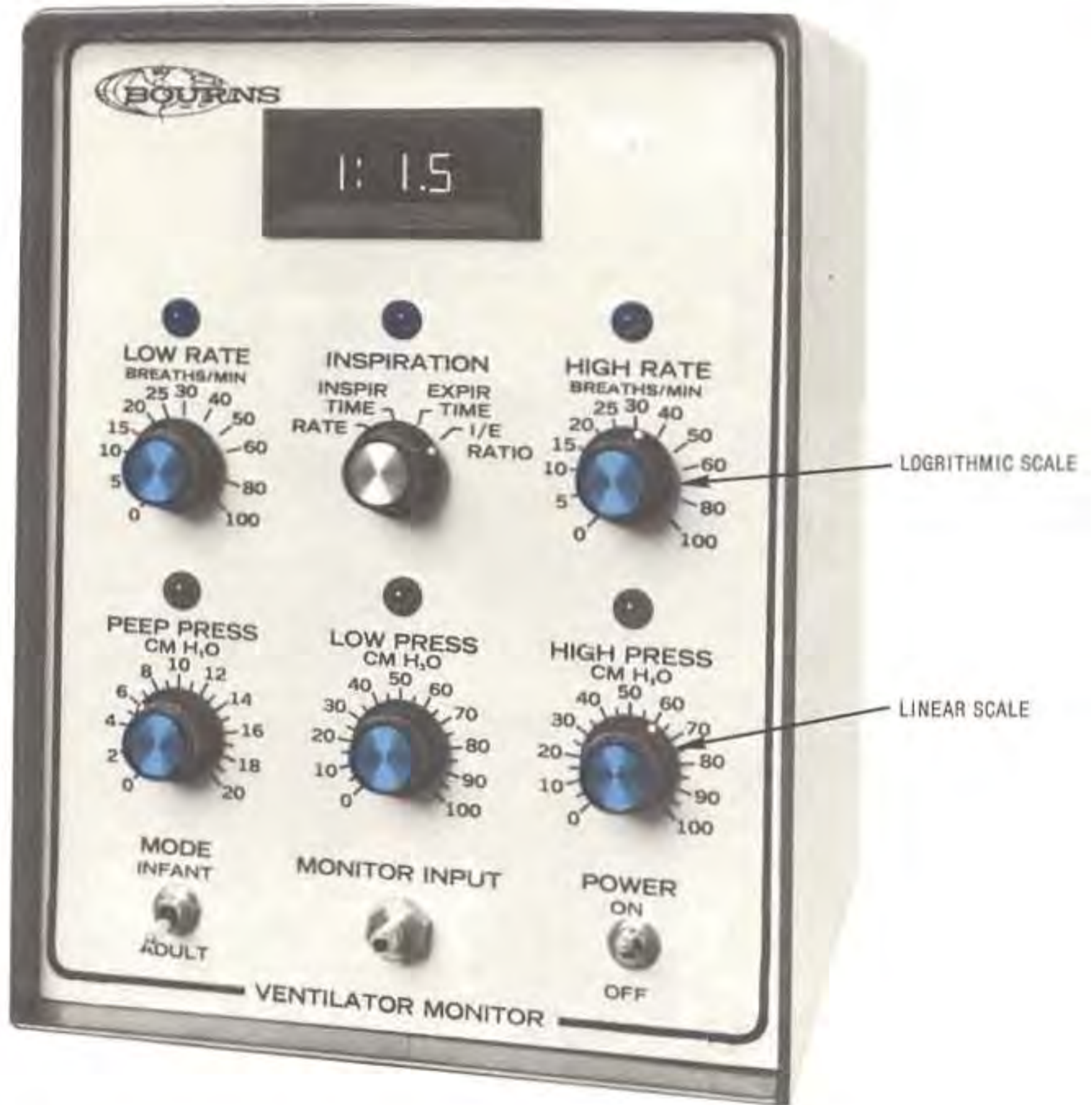
Fig. 3-24 Typical screened or engraved dials for single turn data input
