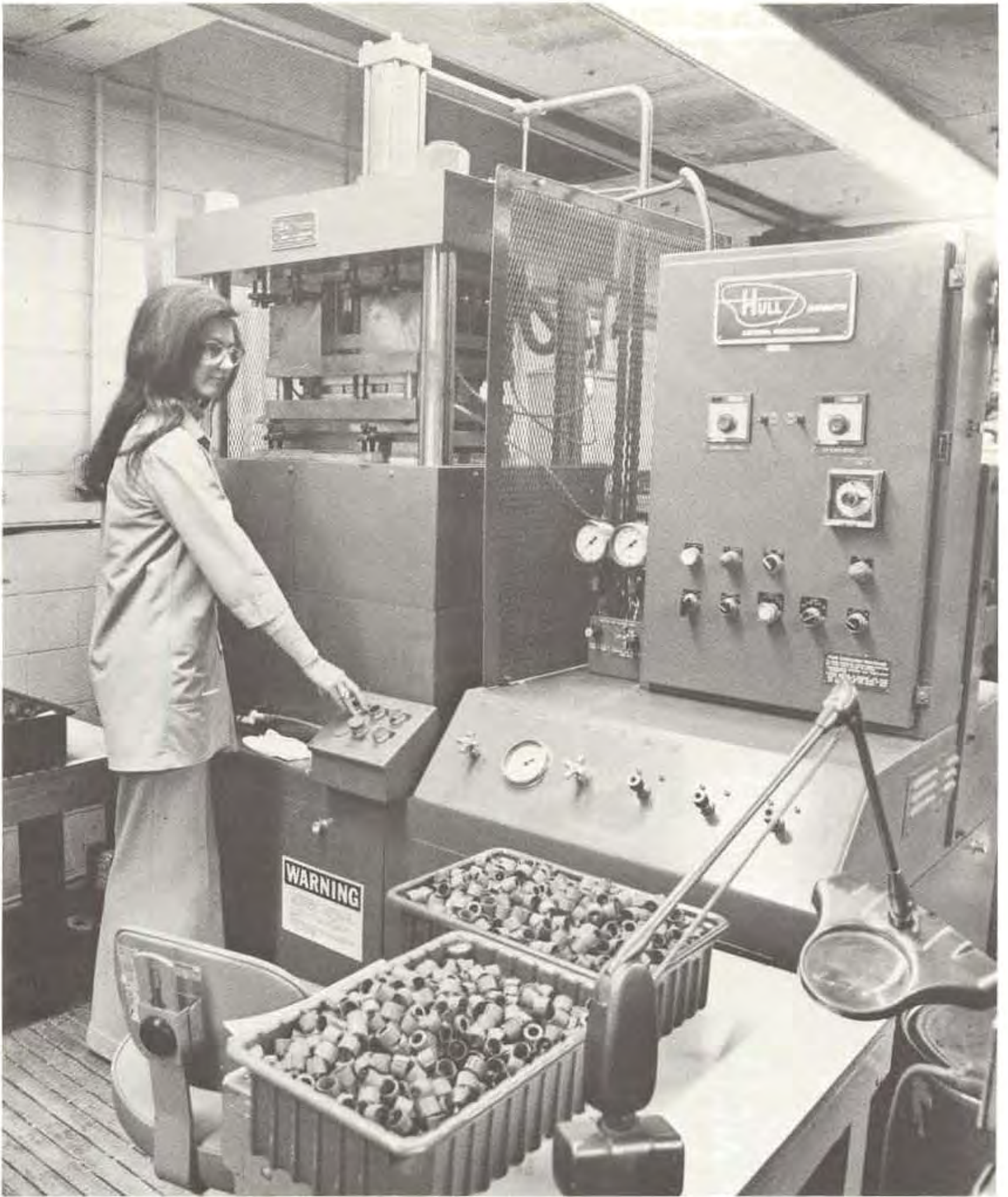
Fig. 7-36 Precision potentiometer housings are molded by equipment such as this press
