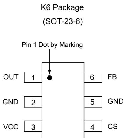
Figure 2. Pin Configuration of AP1680 (Top View)
