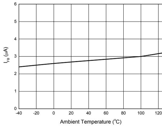
Figure 7. I<sub>FB</sub> vs. Ambient Temperature
