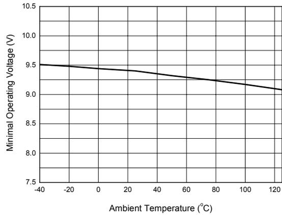
Figure 5. Minimal Operating Voltage vs. Ambient Temperature
