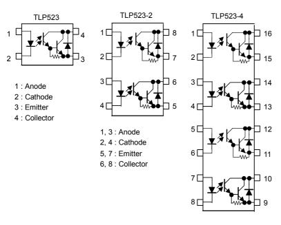
1, 3, 5, 7 : Anode 2, 4, 6, 8 : Cathode 9, 11, 13, 15 : Emitter 10, 12, 14, 16: Collector Unit: mm
