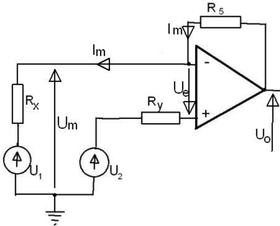
$$U_1 = \frac{U * R_3}{R_3 + R_4} \quad R_x = \frac{R_3 * R_4}{R_3 + R_4}$$
