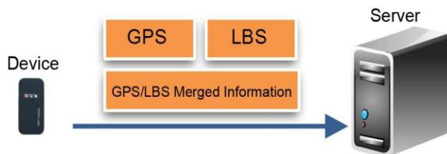
3. In order to protect the validity of connections, the device will send status information to server at fixed intervals then the server return responding package switching for confirmation.
