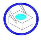
2 Neither directly touch the gel surface with the hand or sharp instrument, it may damage its internal circuit.
