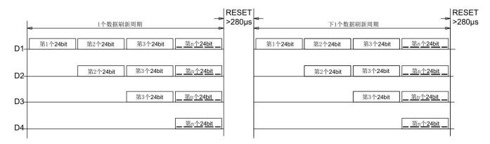
Note: The data of D1 is sent by MCU, and D2, D3, D4 through pixel internal reshaping amplification to transmit.
