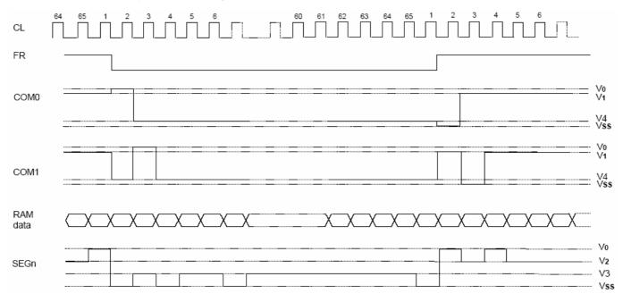
When multiple NT7534 chips are used, the slave chips must be supplied with the display timing signals (FR, CL,/DOF) from the master chip. Table 5 shows the status of the FR, CL, and /DOF signals.
