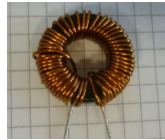
Fig. 5. Inductor: Core 77310-A7 (KoolMμ material), N=57 turns.
