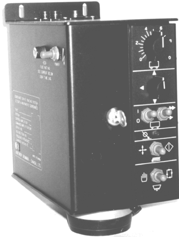
Figure 1-1 HL-90 Drive Tracing System
