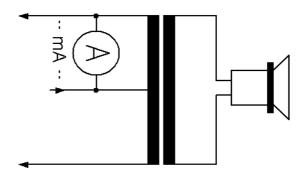
The meter is set to the appropriate ampere scale (200mA), and the probes are connected parallel to one half of the output transformer - as a rule, the center lead and one of the side leads.
