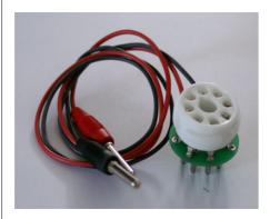
Such an adapter also measures the voltage (voltage drop over the measurement resistor) which is equivalent to the cathode current. In addition, there are adapters that measure the current directly. These adapters, however, can under certain circumstances cause problems, usually instability in the amplifier, and as such are not recommended.
