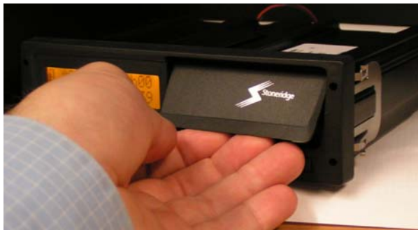
3. Hold the fascia at the bottom where it is tilting outwards.
