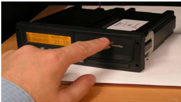
1. Gently press the fascia in the middle near the top of the VU.
