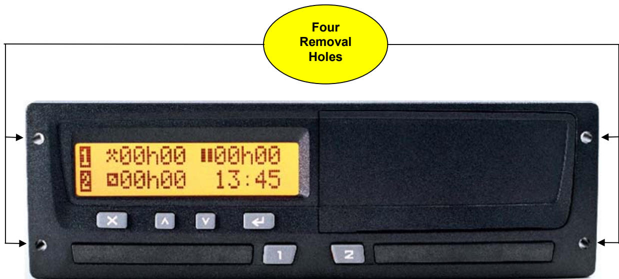
Figure 15 Position of VU Removal Holes
