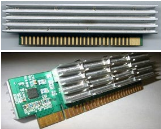
Figure 12 Heatsinks attached to multiple devices
