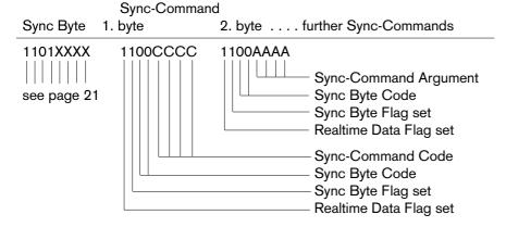
The first Sync-Command byte contains the Sync Command Code in bits 0 to 3. The second byte holds the argument in bits 0 to 3 also.
