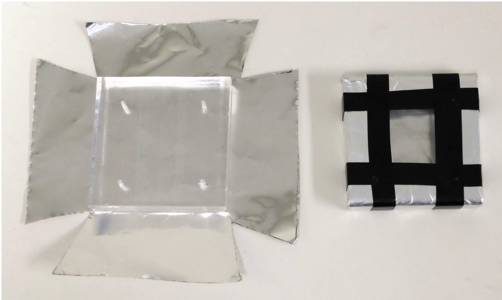
Figure 6: Left: The machined scintillator sitting on top of the reflective foil. Right: the covered scintillator with a 2 \times 2 cm opening for the SiPM.
