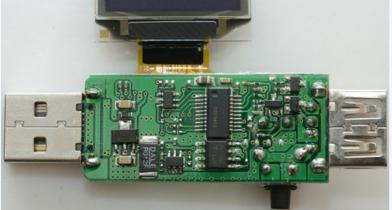
This design looks very simple. It has a voltage regulator, a R012 for current measurement, a processor, a EEPROM and some transistors for turning the output on/off and two 6 pins high precision ADC's.
