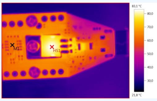
M1: 62,6°C, HS1: 83,1°C The transistor is not very hot for a transistor.
