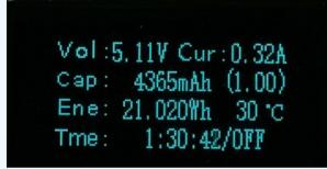
This screen is basically the same as the first, just with labels for the sums and less resolution on voltage and current. The (1.00) shown is a scale factor that can be adjusted in the configuration. Press the button 5 times to define a maximum charge time (AO is auto off), wait to save.
