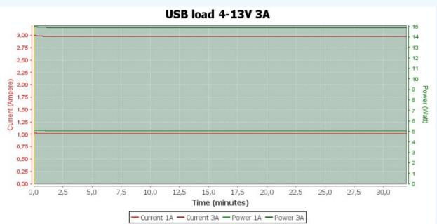
The 3A trace is maximum power for the load, except for the initial drop it stays very stable.
