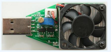
The two chips on this side is 5 volt regulators, probably one for the fan and one for the electronic. The adjustment is a multiturn trimpot with a handle on it. Above the text "POWER" is a red led.
