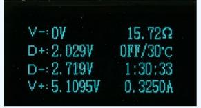
Next screen show voltage on both power and data pins, a calculated resistance of the load, internal temperature, time and current.
