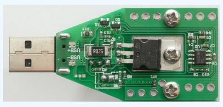
The load transistor is a NPN darlington transistor rated for 65 watt. The R025 is the resistor used to measure the current accross. The actual regulation is done by U2 (LM358 OpAmp), this also handles the temperature control and control Q0 that turns the fan on/off. U1 is a reference used for the current measurement.
