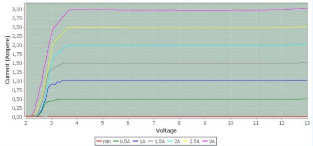
The load is rated from 3.7 volt to 13 volt, the minimum voltage looks correct. The load is fairly stable over voltage, but there is a small change during startup (I did all curves from 13V to 0V).
