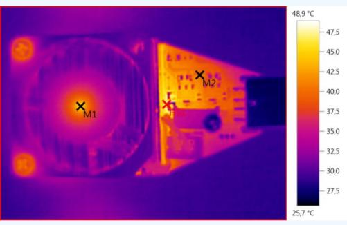
M1: 43,7°C, M2: 40,6°C, HS1: 48,9°C The fan keeps the temperature down, this is from the 1A test.
