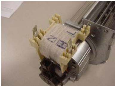
Figure 18 Tape on cooling fan windings marked to designate terminals
