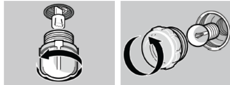
Figure 11 Round halogen ceiling lamp (L); traditional lamp with 40W or 25W appliance bulb (R).
