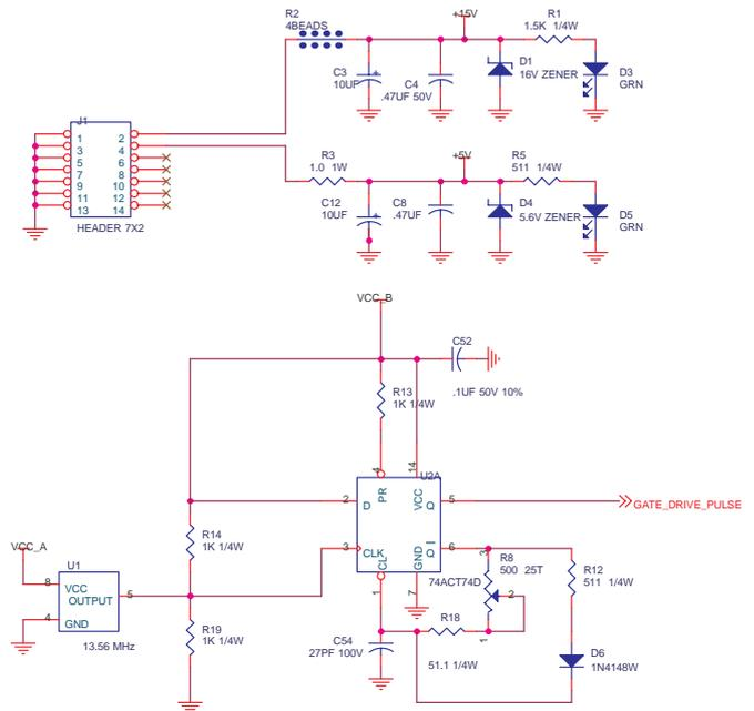
Figure 2: PRF-1150 DC and Gate-Drive Schematic
