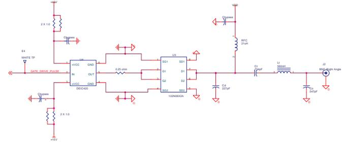
Figure 7: 1KW Class E Functional Diagram
