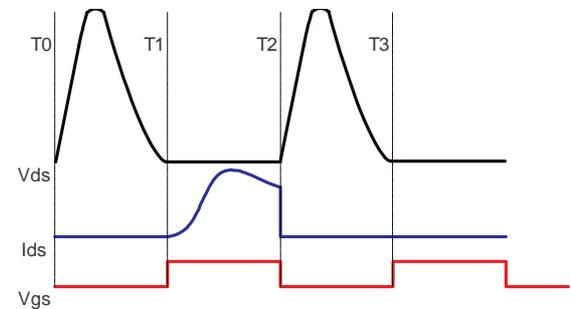
Figure 8: Ideal Class E Waveforms
