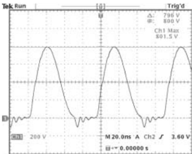
Figure 11: Drain Waveform @ U3, Drain, 1KW output power
