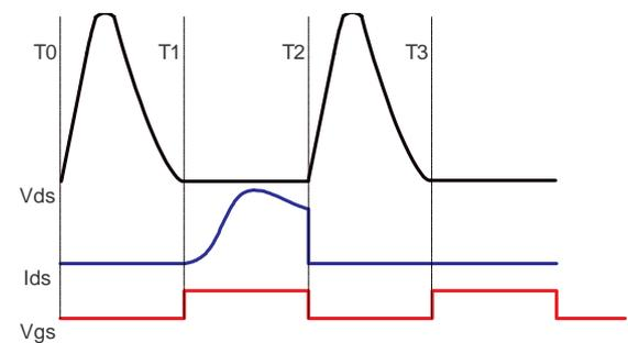
Figure 8: Ideal Class E Waveforms
