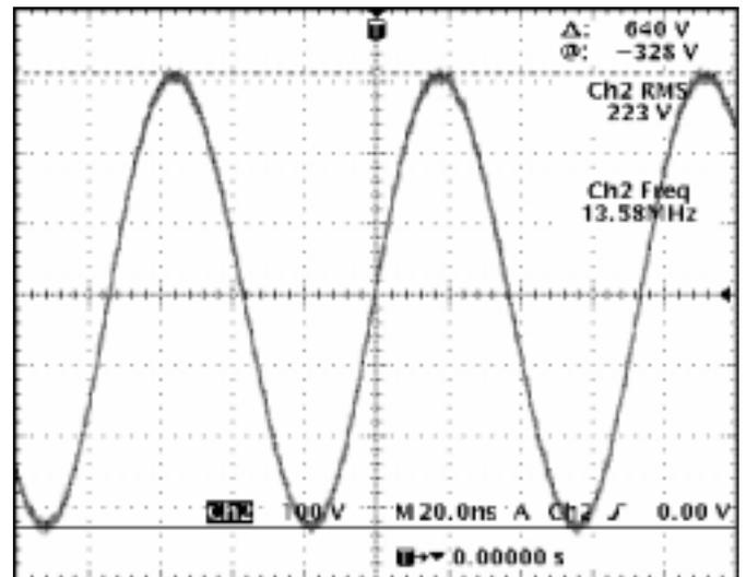
Figure 12: RF output Waveform J2, 1KW output power
