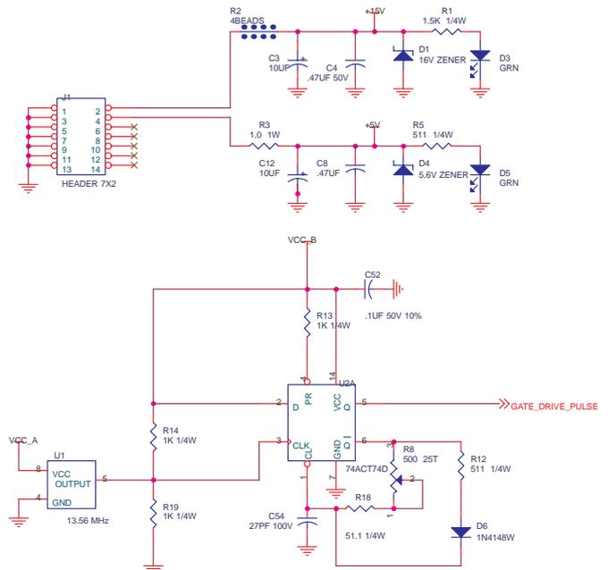
Figure 2: PRF-1150 DC and Gate-Drive Schematic
