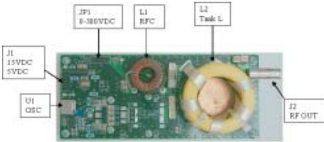
Figure 5: PRF-1150 Left Side Top View
