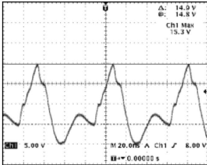
Figure 10: Gate Drive Pulse at U3 gate
