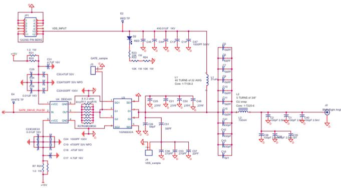
Figure 3: PRF-1150 RF Section Schematic
