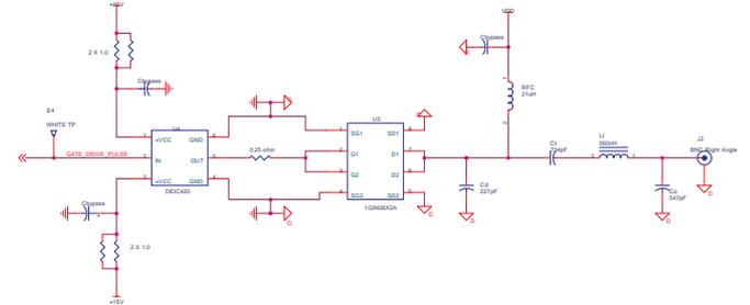
Figure 7: 1KW Class E Functional Diagram
