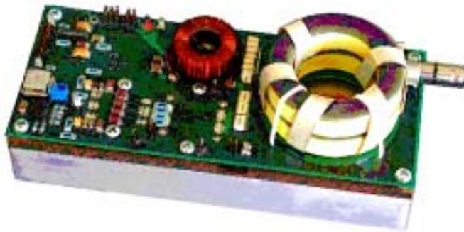
Figure 1: PRF-1150 1KW RF Generator Module
