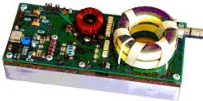
Figure 1: PRF-1150 1KW RF Generator Module
