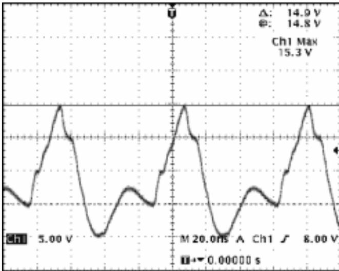
Figure 10: Gate Drive Pulse at U3 gate
