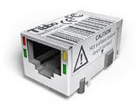
The EM202 is a "RJ45 form factor" Ethernet Module for onboard installation. Module hardware includes one 100BaseT Ethernet port (standard Ethernet magnetics and RJ45 connector are integrated in the EM202), one serial port (CMOS-level), and an internal processor, whose firmware acts as a bridge between the Ethernet and serial ports.
