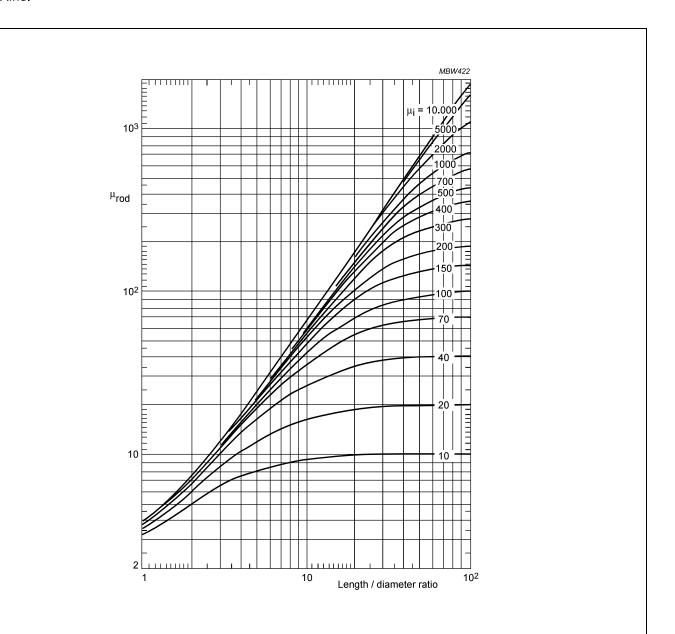
Fig.64 Rod permeability ( $\mu_{rod}$ ) as a function of length to diameter ratio with material permeability as a parameter.
