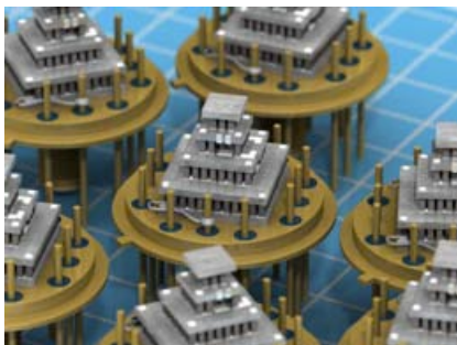
4-Stage TE Coolers on TO-8 Headers Mounting by lead-free Soldering
