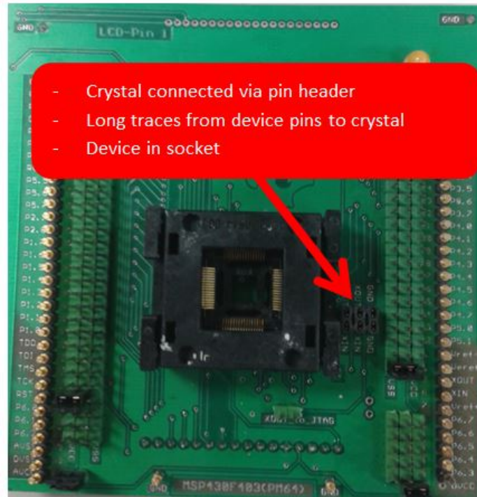
Figure 11. Nonoptimized PCB for General Test Purpose
