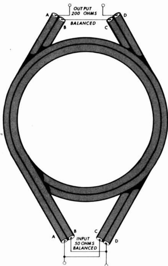
fig. 6. A 50- to 200-ohm balanced-to-balanced transformer made from two 127-cm (50-inch) 100-ohm lines each consisting of two 50-ohm lines in series. The 100-ohm lines are connected in parallel at the input and series at the output. Performance data are shown in table 2.
