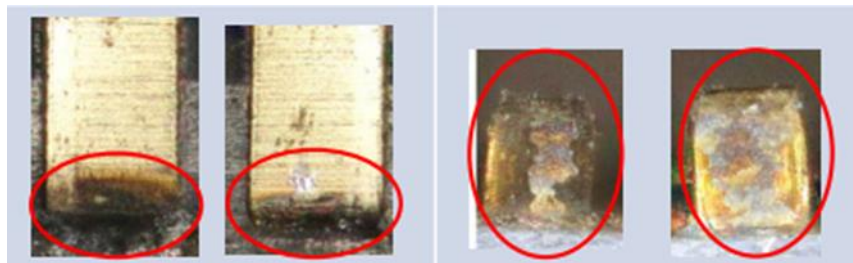
Figure H-1 Arcing Damage to USB Type-C VBUS Contacts
