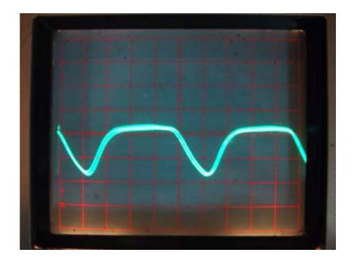
Vertical scale has 0 volts at the baseline and 1kV per division. Horizontal scale is 2mS per division.
