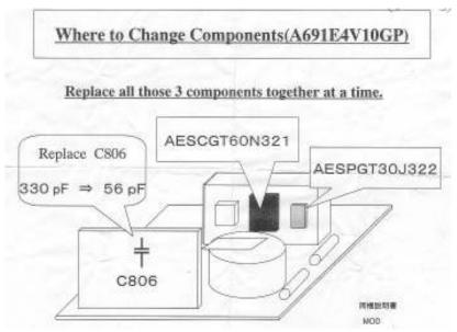
A kit is available consisting of two replacement IGBT's and a replacement capacitor. The GT60N90 has been replaced by a GT60N321 which has a 1kV rating vs. 900V. The smaller GT30J322 is unchanged, although a replacement is supplied in the kit (perhaps this is a post-blowup kit!). Also, a 330pF capacitor on the control board is replaced with a 56pF. Perhaps it would be wise to alter the value of that capacitor anyway, even if the bigger IGBT is not fitted.
