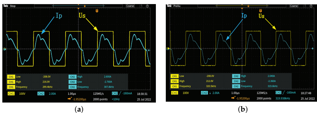
Figure 7. Voltage and current waveforms at inverter output under different frequencies. (a) f = 300 kHz. (b) f = 320 kHz.
