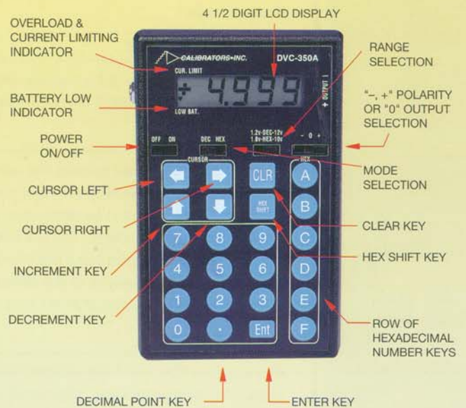
Figure 2. DVC-350A Keys, Indicators and Switches
