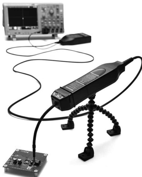
Figure 9x.95. Tektronix IsoVu probing system: completely isolated, with power and signals over fiber. (Copyright© Tektronix. Reprinted with permission. All Rights Reserved.)
