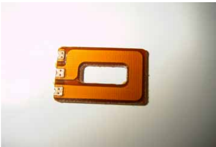
Figure 19: HVPF high voltage planar capable of 2500 Volts
