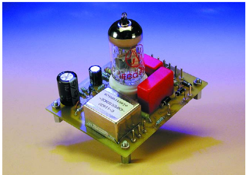
Figure 7. Circuit board layout for ECC83 (board available from Experience Electronics).
