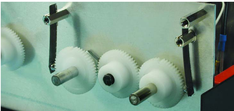
Figure 3. The balance potentiometers are coupled by a pair of gearwheels. The centre-to-centre spacing is 25 mm.
