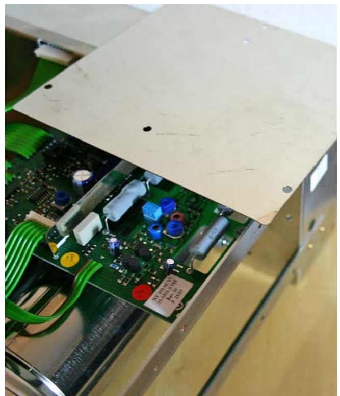
Cabinet capacity replacement
