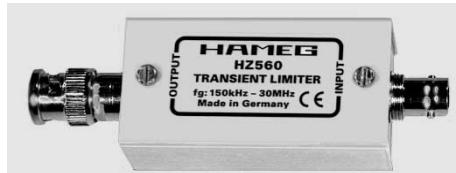
The **HZ560 (Transient Limiter)** protects the input circuit of spectrum analyzers and measurement receivers, in particular in combination with the use of a **Line Impedance Stabilization Network** (i.e. **LISN HM6050**)
